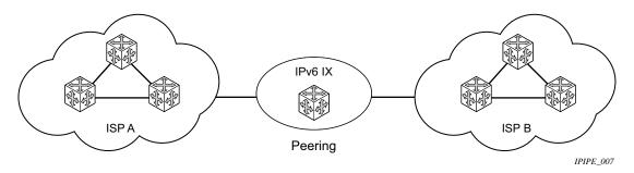
Figure 3: IPv6 Internet Exchange
